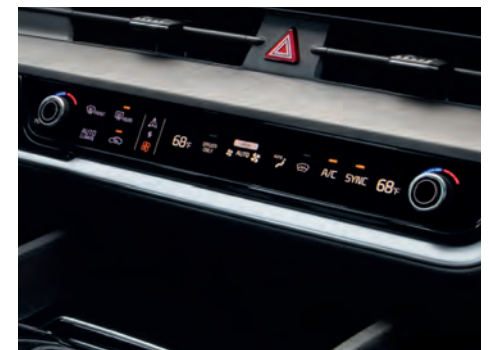
Infotainment/climate switchable controller share the same LCD softkey keyboard.
