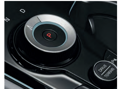
Quick-shifting electronic Shift By Wire (SBW) technology and standard Drive Mode Select (DMS) that adjusts transmission, throttle, and steering response.
