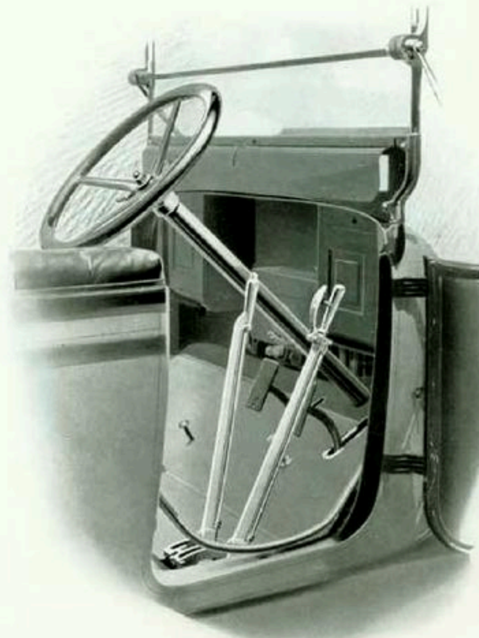
Control Levers are inside with ample clearance
