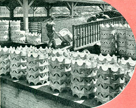
Forgings for crankcase sections for Pratt & Whitney aircraft engines here are shipped from a Chevrolet aluminum forge plant.
