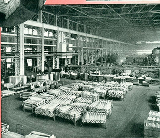
Aluminum pistons, here being burred after forging, are made in vast quantities at another aluminum forge plant.
