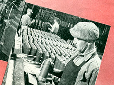
Between these rows of multi-operation machines, armor-piercing shot bodies are sped on a sloping conveyor, progressing toward an inspection station.
