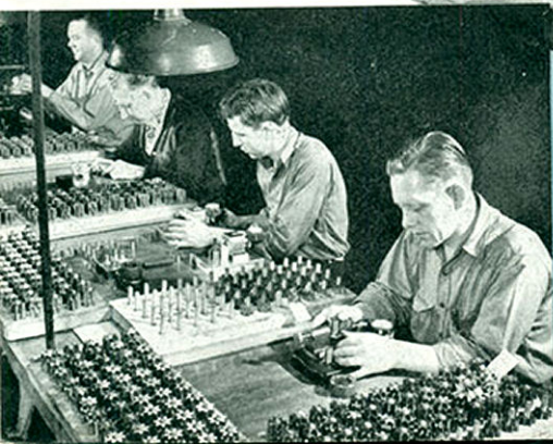
← So finely finished are these Pratt & Whitney engine gears, inspectors keep hands oiled with lotion so that fingerprints will not etch into the surfaces of the gears.
