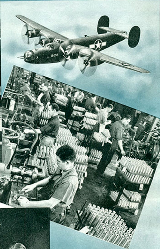
▲ These machine operators are machining valve tappet guides for the Pratt & Whitney aircraft engine in a Chevrolet manufacturing plant.
