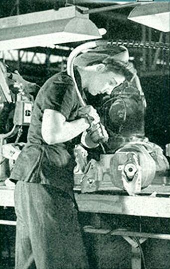
▲ A striking camera study is this picture of a girl employe burring cylinder heads for assembly in Chevrolet-built Pratt & Whitney engines.
