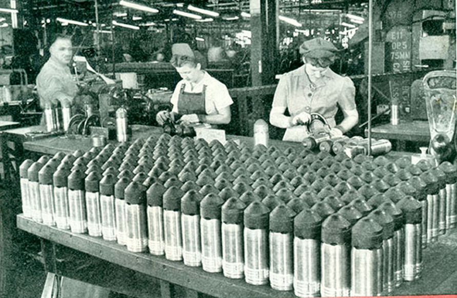
Both 75-mm. and 3-inch armor-piercing shot are produced in volume by Chevrolet. These girls inspect the completed shot, now ready for painting.
