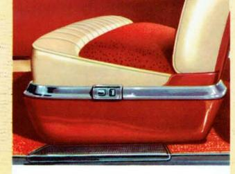
New 4-way power seat control moves front seat up, down, back or forth . . . at a finger touch you can position yourself for safest, most comfortable driving!
