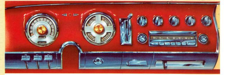
Safety keynotes Chrysler's new dash panel styling. Large dials straddling steering column can be read at a glance; controls and switches are within instant reach . . . and, for the first time, the hand-brake is mounted on panel to the left of the dials.
