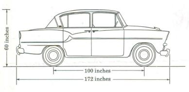
Overall length . . 172 inches Wheelbase . . . . 100 inches width . . 67 inches Tread, front . . . 52 inches height . 60 inches rear . . . . 54 inches Curb Weight . . . . 2700 lbs.
