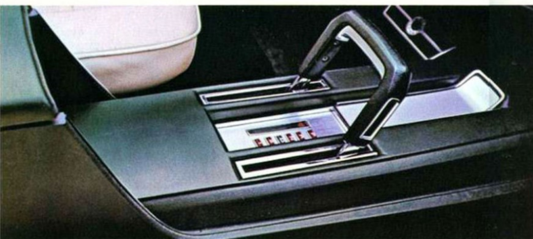
Select Shift. This is Mercury Meteor's two-in-one shift. It's a manual and an automatic at the same time. You can put it in 'Drive' and forget it, or shift through the gears by hand. It's the perfect "his"
