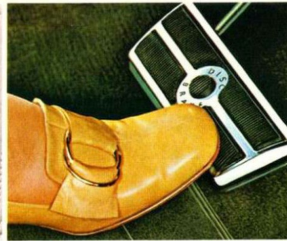
Power Disc Brakes. If you drive in mountainous terrain, or stop-and-go traffic, you'll appreciate the extra stopping ability of power brakes (Disc front, Drum rear). More resistant to fade.
