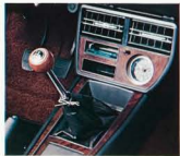
Celica ST standard 4-speed all-synchromesh transmission.
