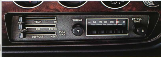
Power-boosted fan-thru ventilation. Heater/defroster with 3-speed blower. AM radio with fingertip on-off button.
