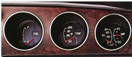
Fuel, temperature, oil pressure and ammeter gauges. All slanted towards the driver.
