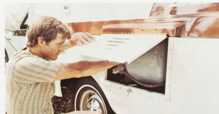
5-gallon LP/Butane tank is located on the outside for easy fill and drain.
