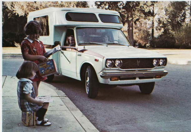
Short wheelbase and recirculating ball steering help make the Chinook an easy-handling vehicle for taking kids to school. Power front disc brakes are standard.
