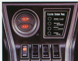
Console-mounted ESP monitors virtually every function of the braking system.
