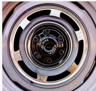
The Wagon has free-wheeling locking front hubs. Standard, as are the power front disc brakes.
