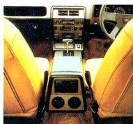
Integrated air conditioning with ducting to rear compartment (floor mounted transmissions only).
