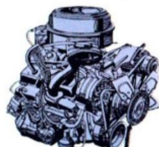
5.0 Liter V8 (305 Cu. In.). Features a staged 4-barrel carburetor and Electronic Spark Control. (ESC not available in Calif.)
