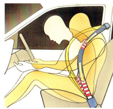
Belt locker device minimises payout of seat belt webbing under extreme conditions.
