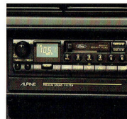
The radiocassette player is protected by a programmed security code rendering the unit useless to thieves.
