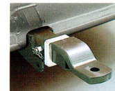
▲ Heavy Duty Towbar (with 1600 kg adaptor) 2300 kg towing capacity with the aid of hitch and load levelling device (purchased separately).
