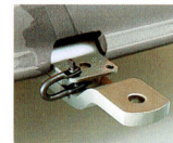
▲ Standard Towbar Rated at 1200 kg for manual vehicles and 1600 kg for autos. Designed to conform to Australian Design Rule (ADR 62) specifications.
