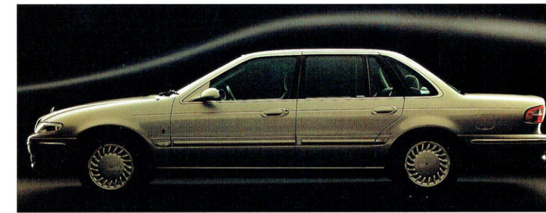
▲ Fairlane's aerodynamic styling contributes to the overall efficiency of the vehicle. The air flow is directed over and around the vehicle to reduce drag. The resultant lower drag coefficient combined with other engineering innovations and refinements promote efficient fuel usage.
