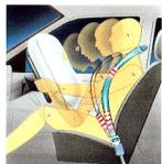
Height adjustable front seat belts, with belt lockers to minimise payout of seat belt webbing in extreme conditions.
