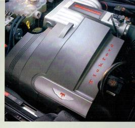
The Tickford-modified 220 kW "Synergy 5000" 5-litre V8 engine delivers power that is smooth and flexible. Numerous enhancements give the engine a pleasing smooth-revving characteristic.
