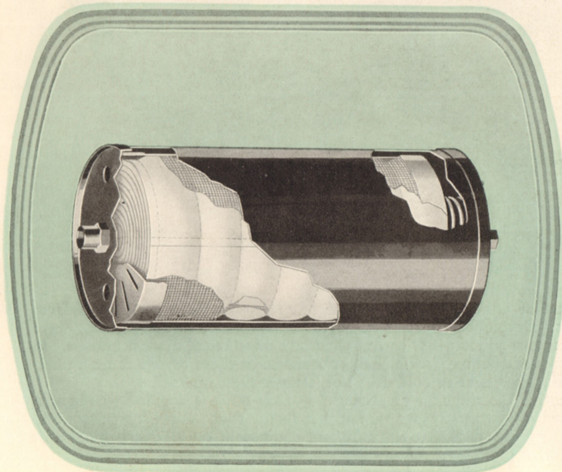
To prevent sediment and water from interfering with carburetor efficiency a gasoline filter, shown to right, has been placed just ahead of the carburetor. The placing of the filter is of particular significance as any scale that may have formed in the piping system is completely prevented from entering the carburetor.
