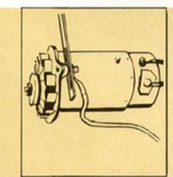
Special electrical equipment is available for the Marshal in addition to the standard 30-amp generator and 60-amp battery provided. Five generator options include 40-amp H.D., 40amp early cut-in, standard 50amp alternator, heavy duty 50-amp alternator and heavy duty 60-amp alternator.
