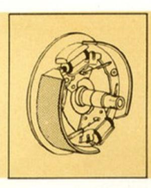
The Marshal's Police Duty jumbo brakes of finned drum construction are the industry's finest . . . provide greater cooling efficiency plus virtually eliminating brake fade. And self-energizing, self-centering shoes with the largest linings of their class give even greater stopping assurance.
