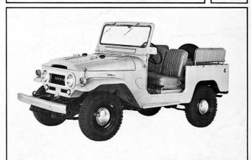
For the man who needs no top, or carries bulky gear, supplies, or equipment, TOYOTA has introduced the new TOPLESS model. In addition to the top, the bows, doors and side-curtains have been removed from this model—thus making it an excellent basic machine for the 4-wheel drive enthusiast who wants to make special adaptations. All stripped parts can of course be ordered and re-installed to produce the normally fullyequipped TOYOTA LAND CRUISER.
