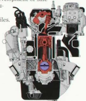
Corona's 4-cylinder, single overhead cam engine (SOHC)
