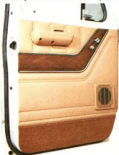
Chateau door panel with woodgrained vinyl center insert and carpeted lower panel and optional stereo radio speaker.
