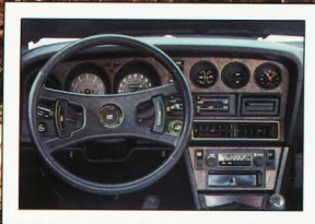
A multifunction dashboard features a tachometer, fuel gauge, speedometer, and odometer. The instrument panel is trimmed in vinyl with simulated woodgrain. Highlights include Liftback's stereo.
