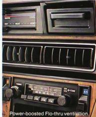
Power-boosted Flo-thru ventilation.
