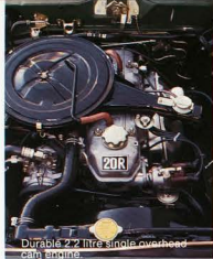
Durable 2219cc single overhead cam engine.
