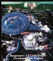
Responsive 2.2 Liter Single Overhead Cam Engine
