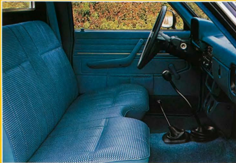
The Sport Truck dash has full instrumentation, padded 3-spoke steering wheel, and easy-care carpeting. Transfer case shift is close to the 4-speed gear lever.
