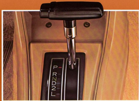
AUTOMATIC TRANSMISSION - It's a durable, smooth shifting 3-speed. Available as an option for people who prefer its convenience.
