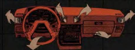
Supra's automatic temperature control air conditioning system maintains the temperature you choose, summer or winter. Balance control directs conditioned air to left or right.
