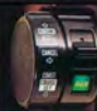
Supra's Cruise Control maintains your pre-set speed on hills as well as level roads. To accelerate, coast, or change settings, simply touch a switch near the tilt steering wheel.
