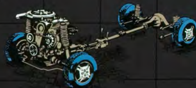
Engine power in the Tercel 4WD Wagons is routed through the transmission and then split between the front and rear drive systems when 4WD is engaged.
