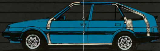
EXTRA BODY REINFORCEMENTS REDUCE NOISE AND VIBRATION
