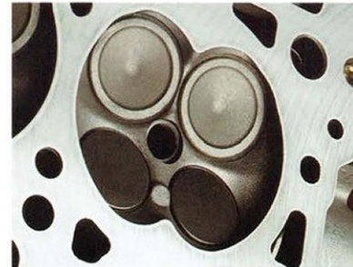
The curved lip around the inlet for the primary intake valve directs the fuel-air mixture as it enters the combustion chamber, causing it to swirl.
