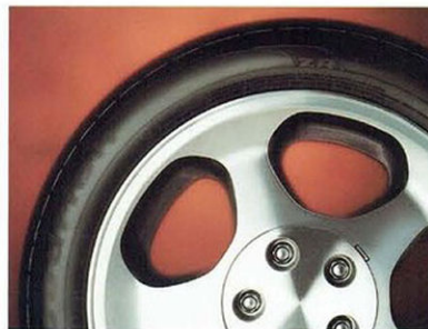
The Cobra's 17.0-inch five-spoke alloy wheels are wrapped with BFGoodrich Comp T/A ZR radials, which are derived from the Comp T/As fitted to SVT's 1995 Mustang Cobra R race car.
