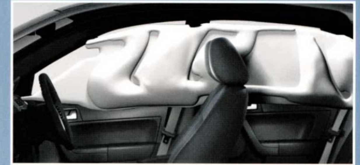
SIDE-CURTAIN AIRBAGS descend from the headliner in the event of a side impact to provide additional protection for front and rear-outboard passengers.
