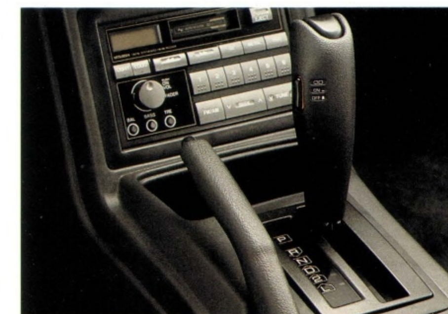
Four-speed automatic transmission features overdrive lock-out control and Power/Economy modes. Standard on GSX, optional on GS.
