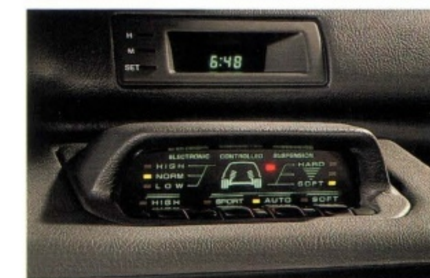
Full-function cruise control (top) is stalk mounted for ease of operation. Active-ECS ™ suspension on Galant GSR features a dash-mounted ride-control center (above) with suspension mode display.
