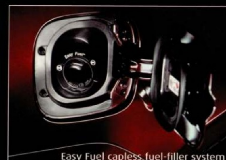
Easy Fuel capless fuel-filler system
