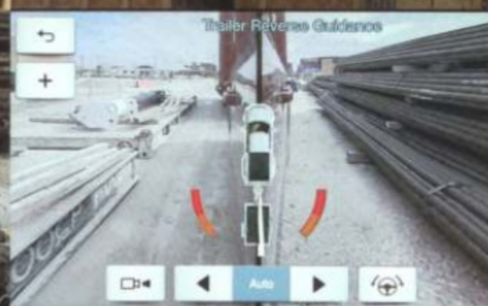
Trailer Reverse Guidance 1 automatically switches between side and rear camera views to show you what is most relevant while backing up your trailer, and provides overlays to guide you.
