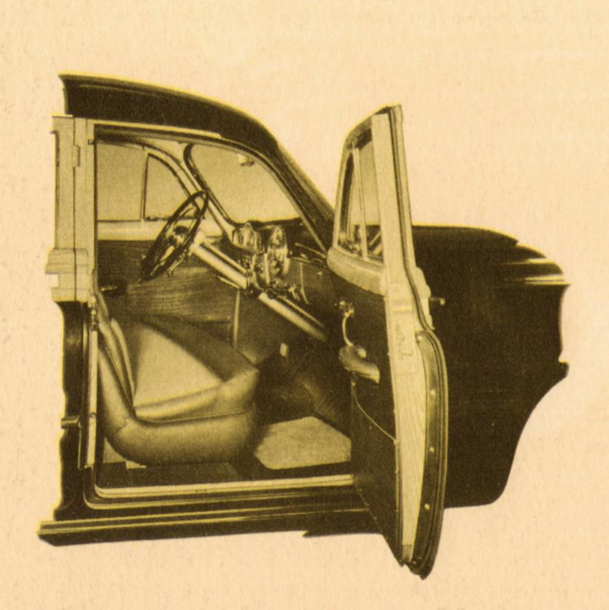
Pontiac's new, wide doors are of rigid steel construction, highlighted by the rich beauty of mahogany panels and hardwood pillars. Doors are counter-balanced for easy swinging and are flush with the floor.
