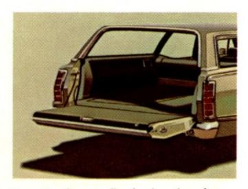
The new 3-Way Tailgate goes one better, it drops flush for loads or swings wide like a door with the window up or down.
