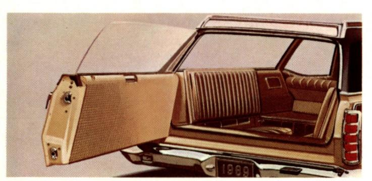
Mercury's, industry leading new 3-Way Tailgate operates three ways to make it easier for cargo or people getting in or out. It drops flat, or opens like a door with the window open or closed. A power rear window is standard on Colony Park.
