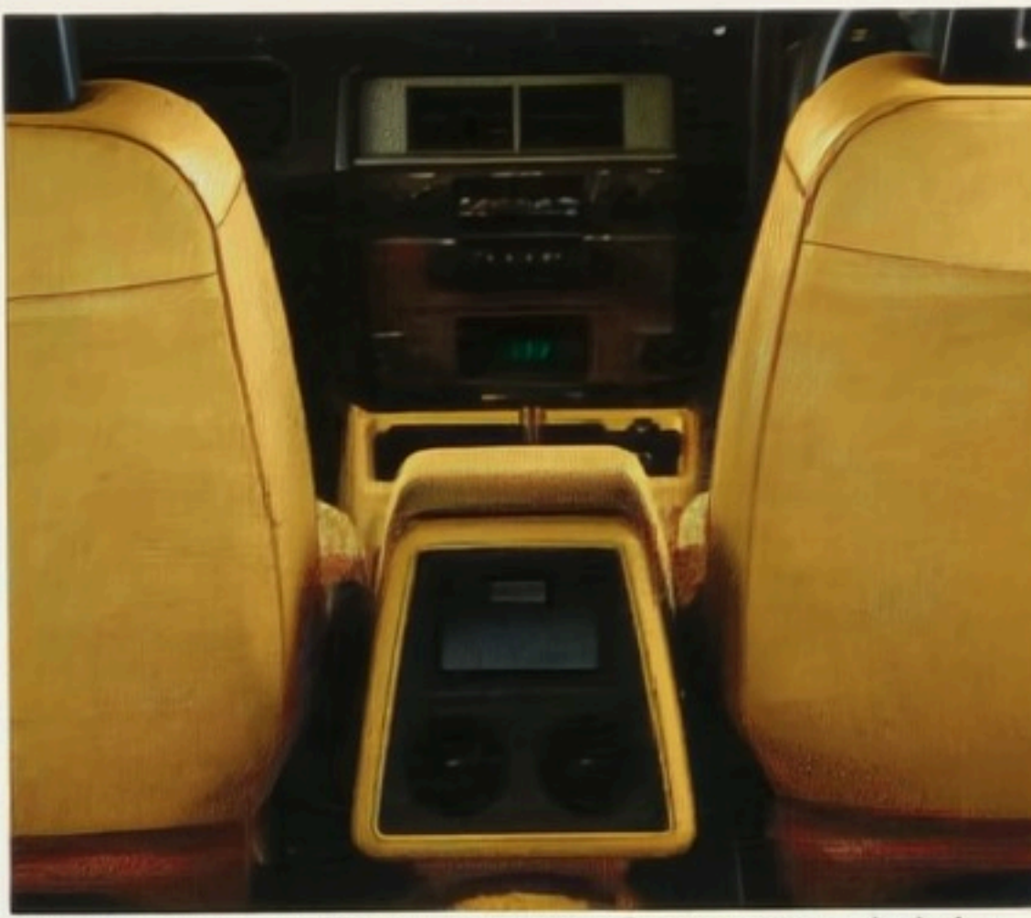
Integrated air-conditioning illustrated in Fairmont Wagon includes ducting to the rear seat passenger area except where a column mounted transmission is fitted.
