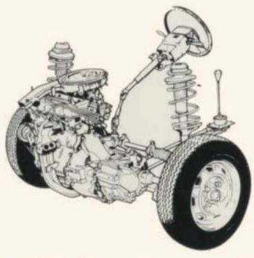
To begin with, being a front wheel drive, the major mechanicals are mounted sideways or transversely, and incorporate engine, clutch, transmission and final drive. This compact unit fits neatly across the engine compartment, leaving space for easy access without taking up a great deal of the car
