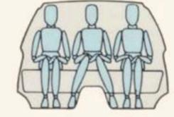
drive car, passenger space is taken up by he driveshaft tunnel. Right, Front wheel drive provides more space and comfort for
