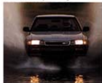
Water tests check for seal tightness.
