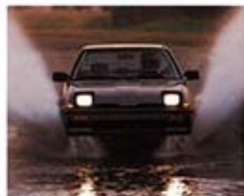
Water tests check for seal tightness.
