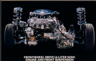
FRONT-WHEEL DRIVE 1.6 LITER SOHC ENGINE AND FRONT SUSPENSION
