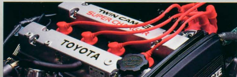
Twin-cam 16-valve performance is boosted by a belt-driven supercharger.
