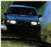
▲ The main trunk at Hallered features a variable-depth water trough, so that brakes can be fully wetted prior to performance and landing tests.
