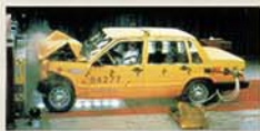
▲ At Volvo's Crash Safety Laboratory (above left), each crash yields roughly 70,000 pieces of information from four accelerometers, force sensors and elongation gauges.
