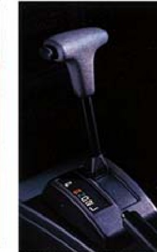
Optional automatic transmission (3-speed on Geo Prizm and Geo Prizm LSi; 4-speed overdrive on Geo Prizm GSi).
