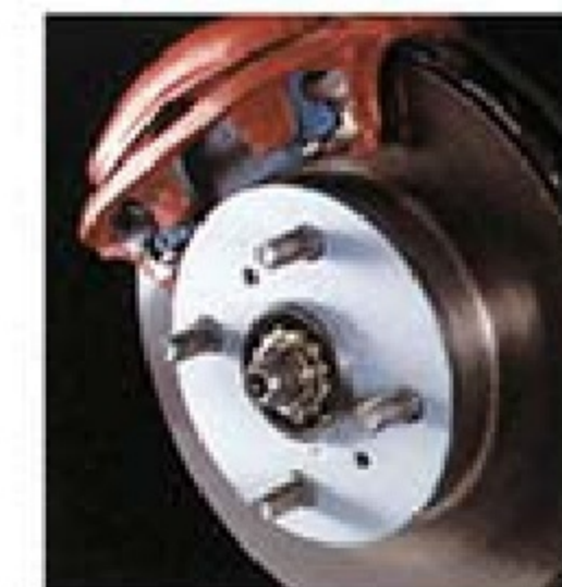
Geo Prizm GSi features standard four-wheel power disc brakes.
