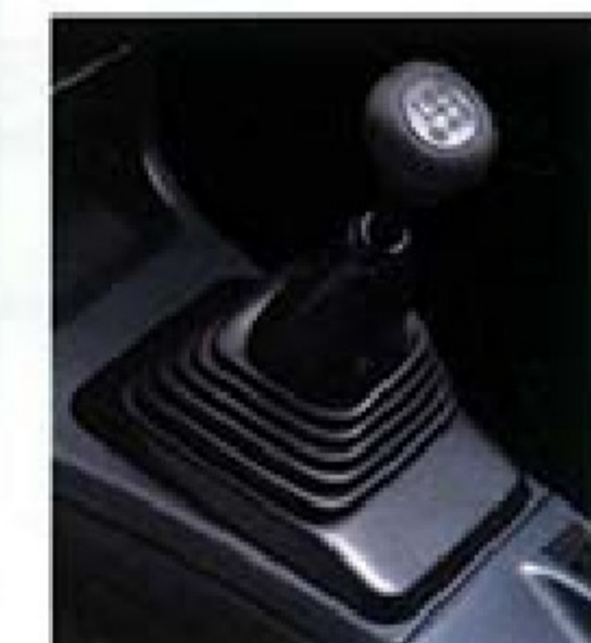
A 5-speed manual transmission with 4th and 5th gear overdrive is standard on all models.
