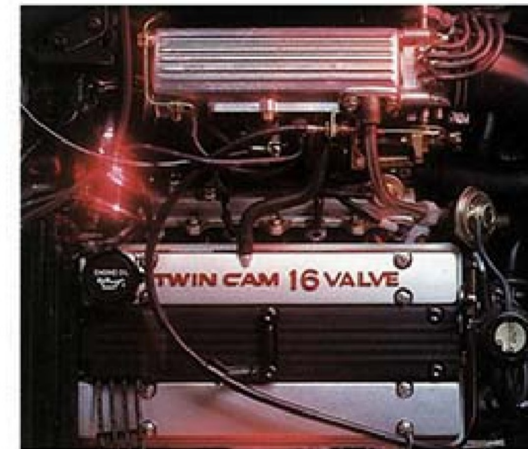
The engine technology that helps make Geo Prizm a smooth, powerful performer includes four valves per cylinder (two intake and two exhaust) for improved volumetric efficiency, a dual overhead camshaft design for weight reduction and faster valve reaction for improved high-RPM performance and Multi-Port Fuel Injection for excellent response and drivability.
