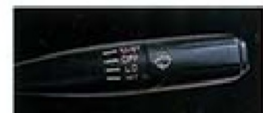
Mist-cycle wipers allow you to adjust wiper speed to match weather conditions.
