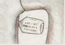
*The stalk-mounted cruise control system includes settings to hold speed, adjust it up or down, or cancel. A light touch of the brake or clutch pedal cancels it also, and it remembers your previous speed.*
