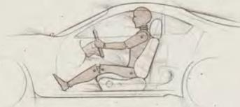
The power driver's sport seat is standard in the new Supra, with leather seat trim optional on both models. The hip point is low with the object being to make the driver a more organic part of the car's control module. The seat has a power slide length that easily accommodates normal to tall drivers.
