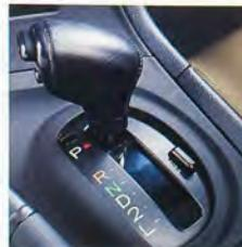
3-liter sports car class. Several methods of exhilarating through the gears are available, all top-notch. Pictured left is the 4-speed electronically controlled automatic overdrive with "intelligence" (ECT-i)\* which varies the shift points according to driving
