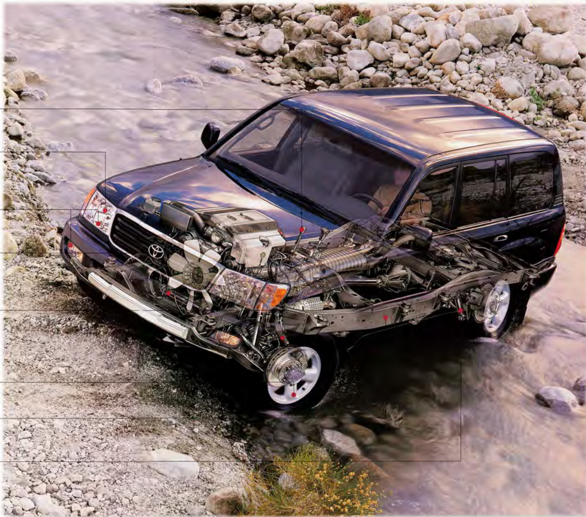
Shown here in Black, Land Cruiser comes prepared for virtually any conditions including wading with wallabies. The driver knows not to enter water deeper than three-quarters tire diameter.
