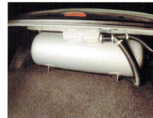
Specially designed LPG tank, fitted so that loss of boot space is kept to a minimum.
