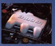
The Malibu LS Millennium is equipped with standard V6 power. The 170-hp 3.1L 3100 V6 generates 190 lb.-ft. of torque, allowing it to respond to every input without hesitation, even at low and moderate engine speeds.
