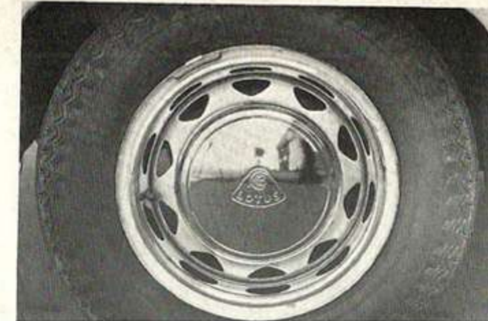
Lotus designed bolt on wheels fitted with radial ply tyres as standard equipment.
