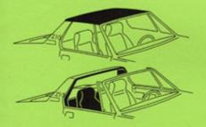
Quickly convertible on account of the ingenious arrangement for storing the removable hard top in the front luggage compartment. The X1/9 has all the attractions of an open two-seater with the comfort and safety advantages of a coupe. The hard top is made of a special light and particularly robust synthetic material - it is retained by means of two over centre clips onto the upper edge of the windshield at the front, and two locating arms onto the roll over bar at the rear.
