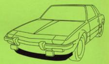
Fitted at the front is an air-dam which both improves road holding at high speed, and channels air into the radiator intake located above it.
