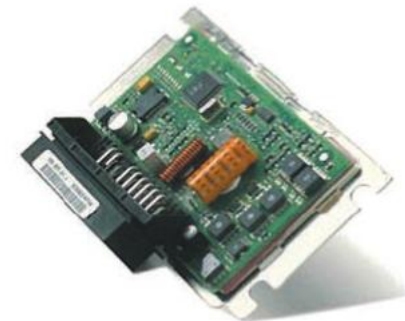
Centralina E-Diff The E-Diff's control unit
